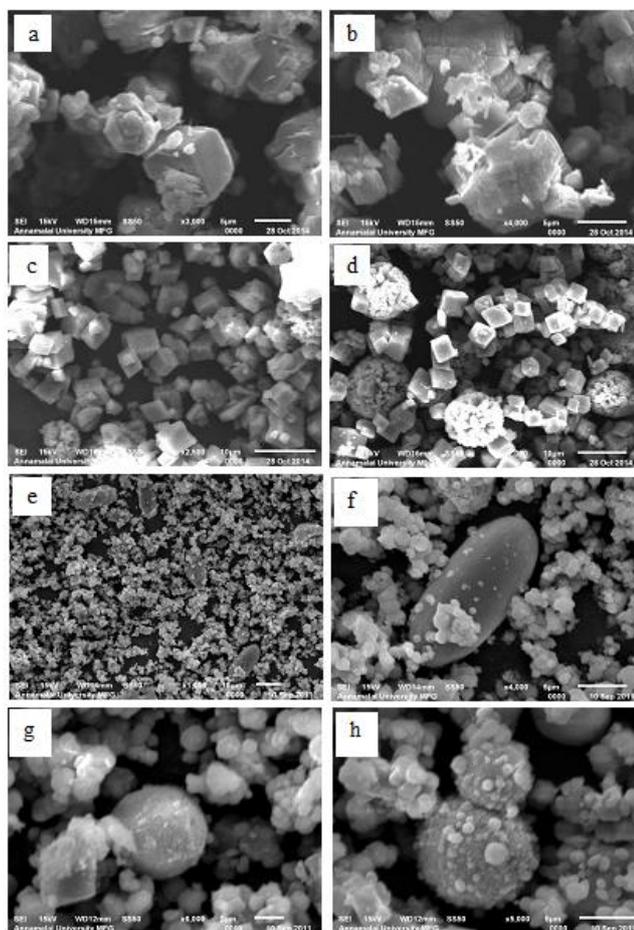
As the temperature is further increased at 80 °C the morphology exhibited marked difference and presence of spherical particles became more prominent. The XRD and FTIR confirmed the presence of aragonite in this sample. There could be larger sized particles with cucumber shape. This could be assigned to calcite. This indicated that the vaterite formed just before has been converted into a binary mixture of aragonite and calcite.
